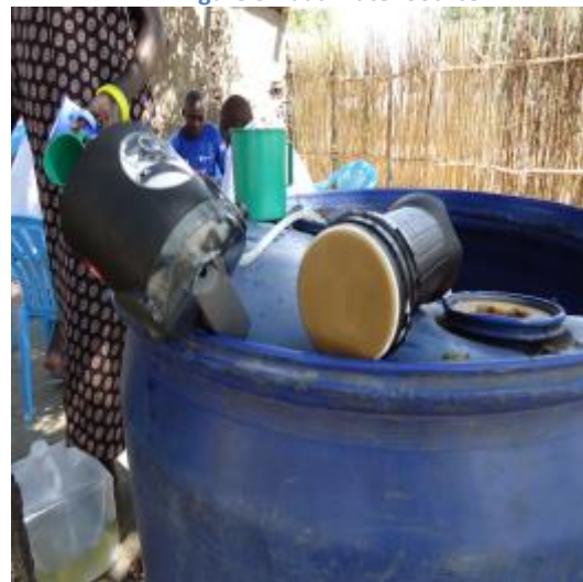
Figure 4 Ceramic filter after filtering 20l of water
