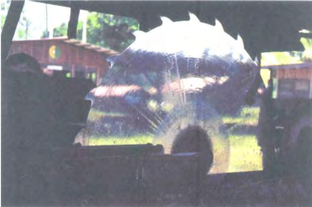
Photo 31: Circular saw headrig (note the wide gullets in saw-blade)
