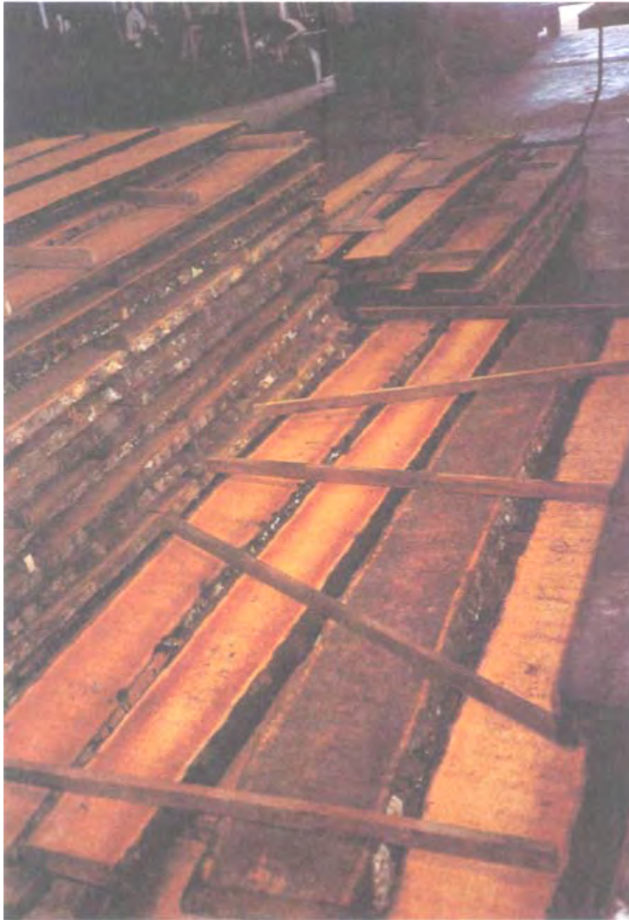
Photo 39: Stacked coconut boards (note fungus-infected board, second from right)
