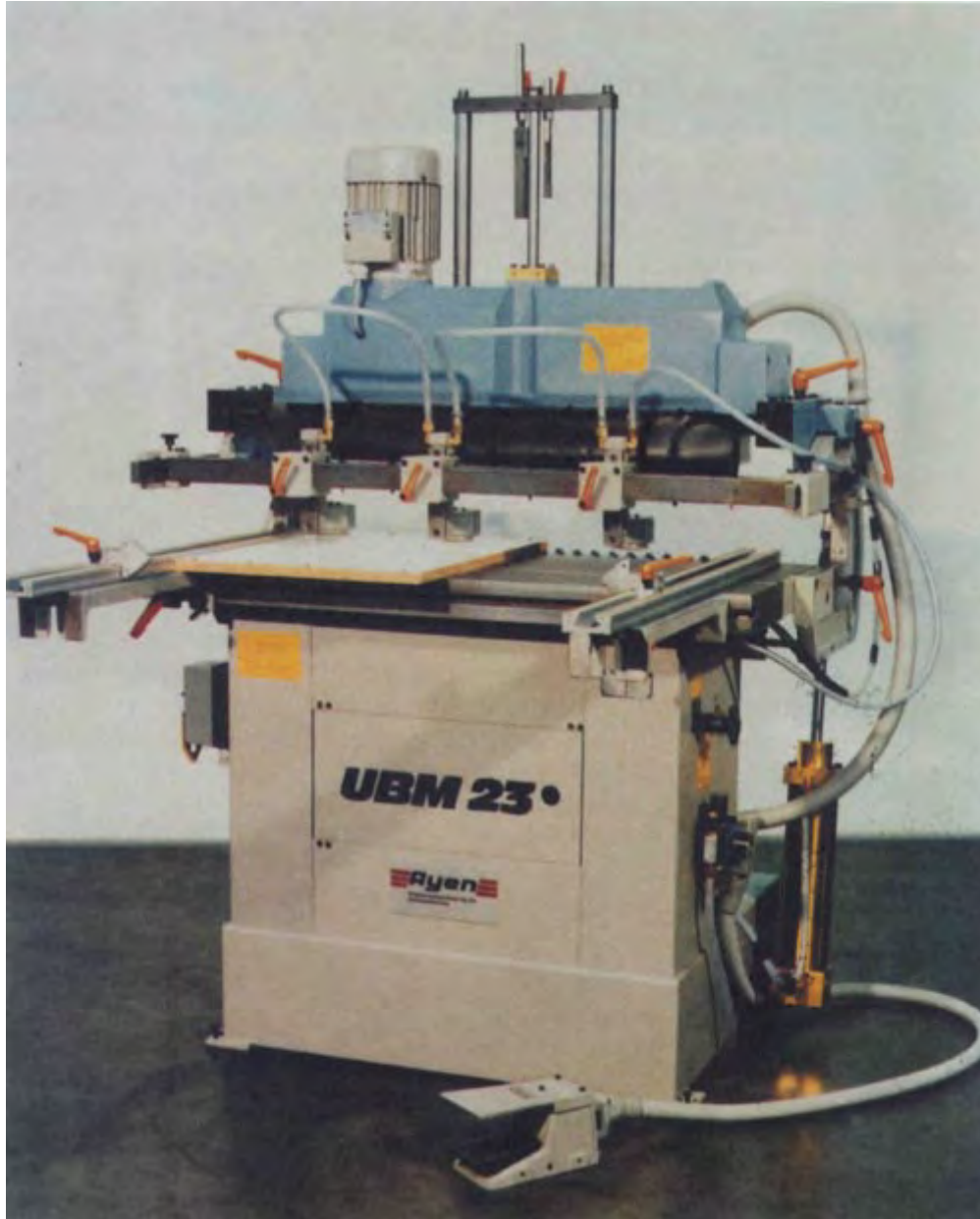
Photo 54: Boring machine with swivellable boring head
