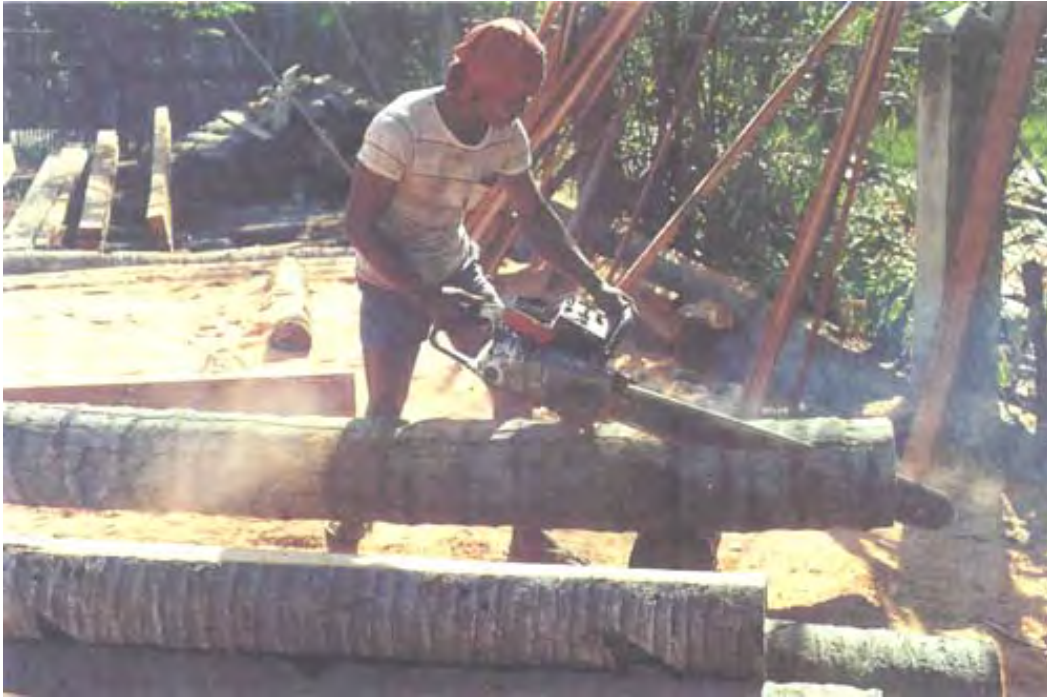
Photo 30: Chain-sawing of palm stems with guide bar
