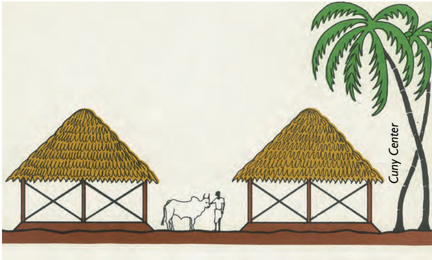
Shelter design elevation showing cross-bracing
