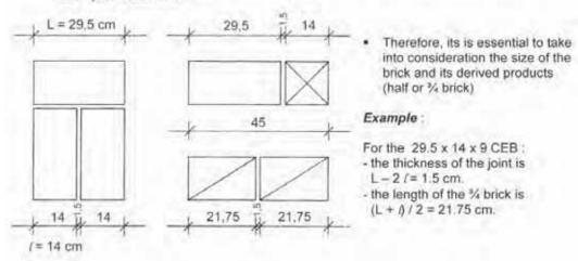
All the bricks are drawn to check the bonding. All dimensions are calculated according to the size of the « brick + the mortar joint ».
