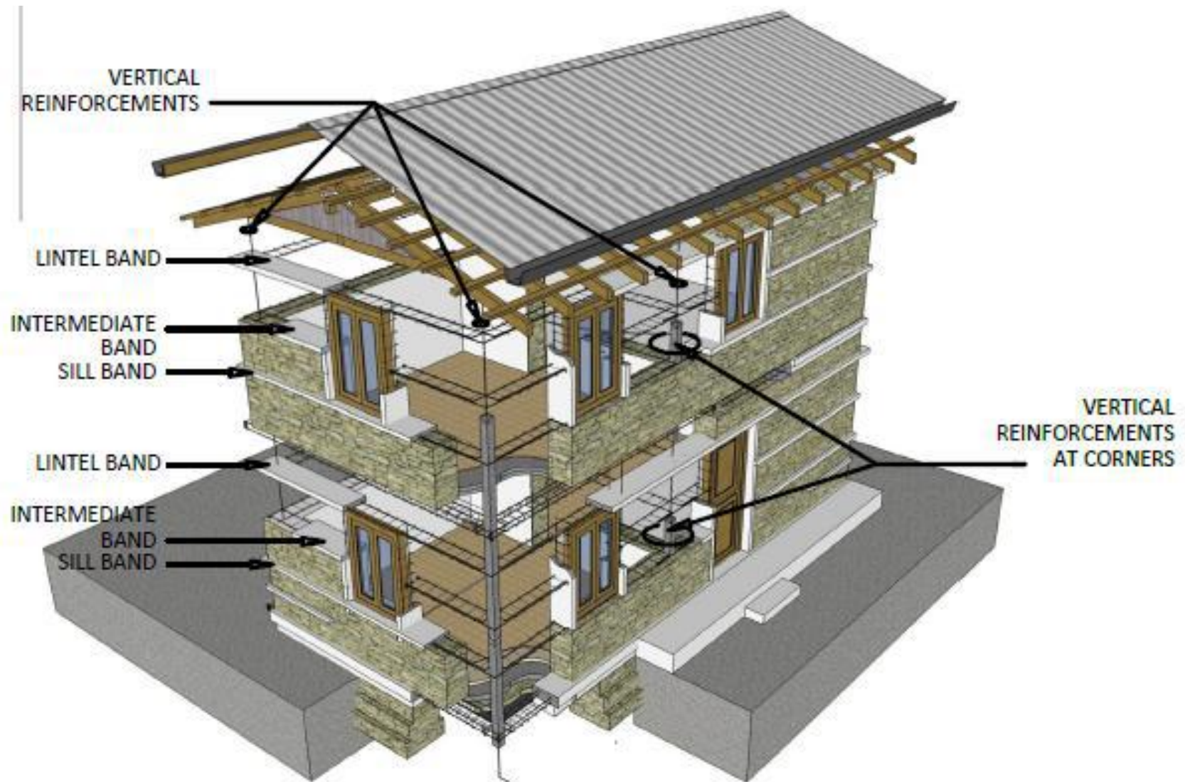
Technology for Earthquake Resistant Building Construction (Two Storied Building, Stone in Cement Mortar)
