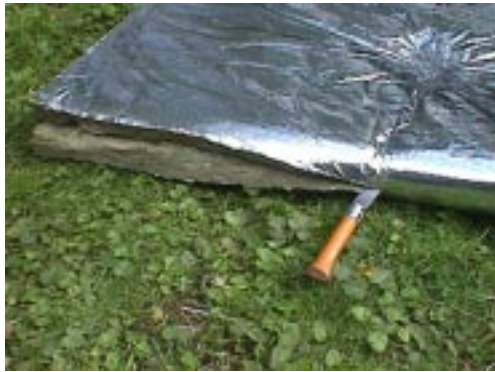
mineral fibre duct wrap is easy to cut but difficult to join
