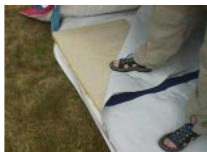
high density mineral fibre batts between two reinforced UNHCR tarpaulins
