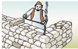
Through stones in stone masonry wall
