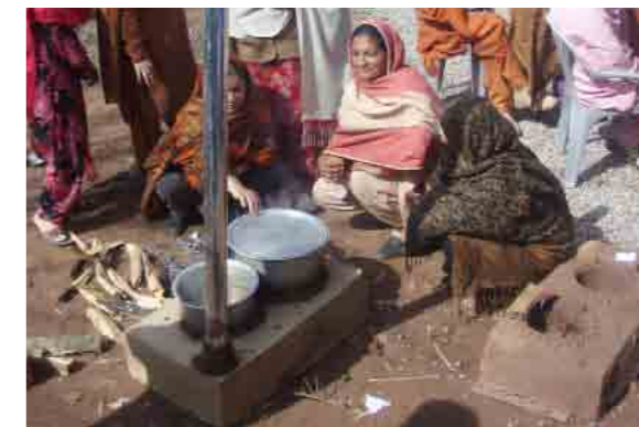
Improved traditional mud stove, training by and for women, low cost, easily to replicate solutions. Improved stove reduced fuel use by an average of 40%.
