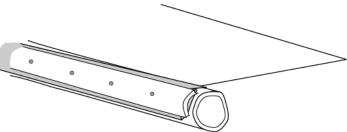
✓✓ plastic sheeting folded over then wired (better) or nailed through section of bamboo
