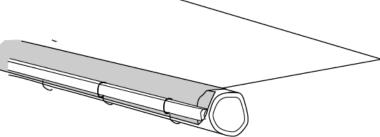
✓✓ plastic sheet folded back on itself, then wire looped around batten passed through hole in the sheet and wrapped around the pole
