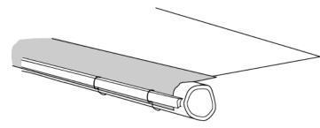
✓ wire looped around batten passed through hole in the sheet and wrapped around the pole
