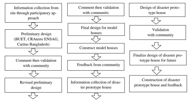
Figure 4. Sequence followed for developing the design of LCH in the project.
