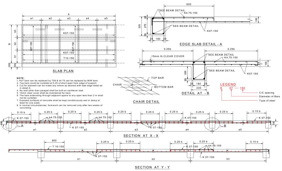
Figure 7.2: Slab Details
