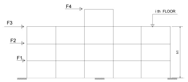
Figure 6.1: Floor Level Lateral Forces
