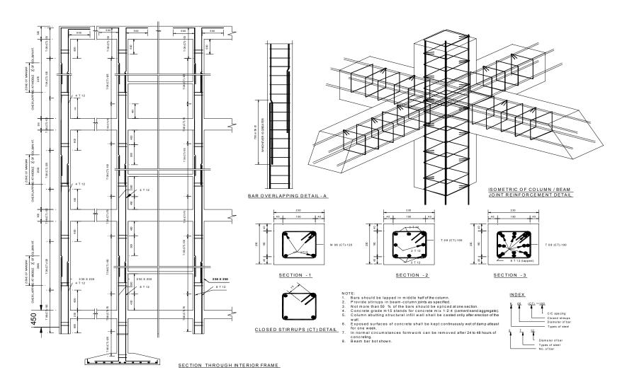
Figure 7.4a: Column Detail (two walls each way / 100 m<sup>2</sup>)
