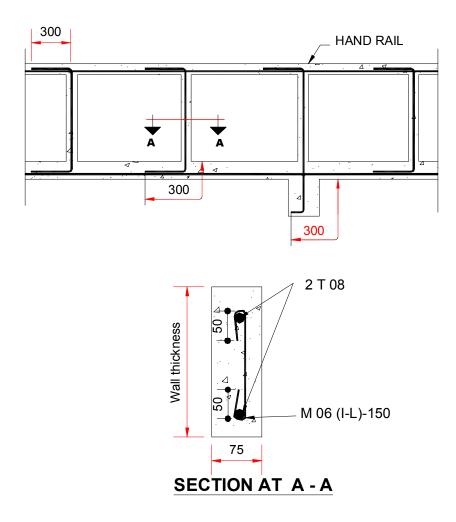
Figure 9.1: Parapet Wall Tie-Up Details
