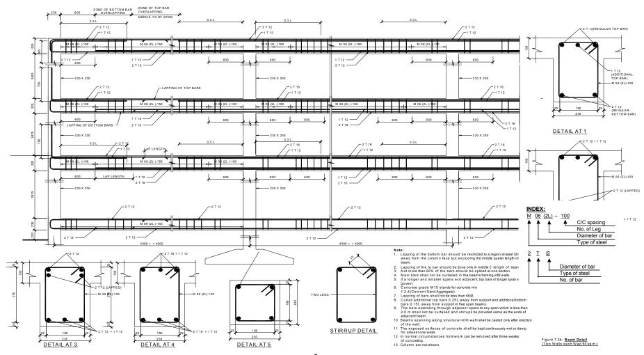
Figure 7.3b: Beam Detail (two walls each way / 60 m<sup>2</sup>)
