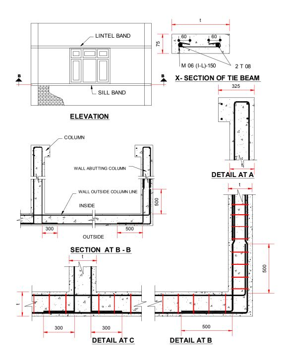
Figure 8.4: Wall Outside the Frame
