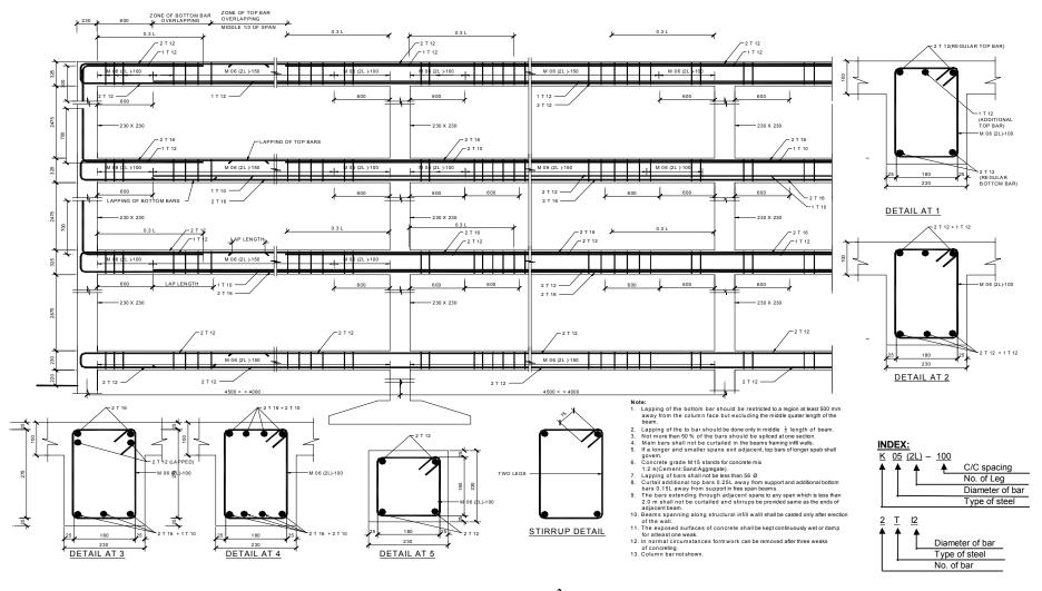
Figure 7.3a: Beam Detail (two walls each way / 100 m<sup>2</sup>)
