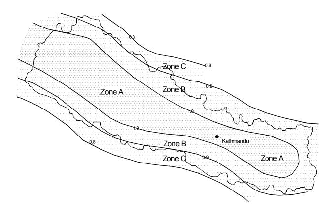
Figure 1.1: Seismic Zoning Map of Nepal for this MRT
