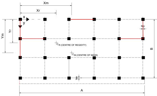
$C_R$  = Centre of rigidity,  $C_M$  = Centre of mass,  $t_{ex}$   $t_{ey}$  = Effective thickness of infill wall along x and y axes respectively
