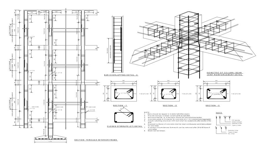
Figure 7.4b: Column Detail (two walls each way / 60 m<sup>2</sup>)
