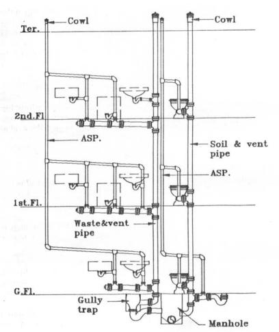
ASP: Anti-siphonage pipe GF.fixtures can be connected directly to GT/MH.
