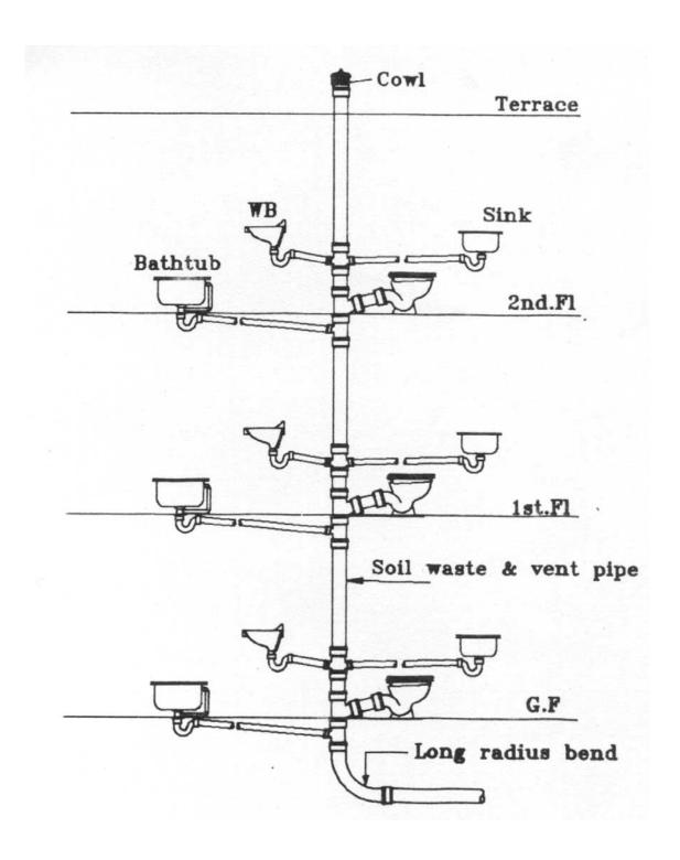
Single Stack System Sewage/Waste Water Collection Illustration B3
