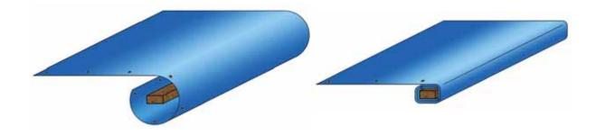
Allow approximately 2 feet (60 cm) of tarp to wrap around the furring strips, so that you have three or four tightly wound layers.
