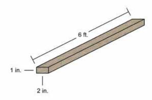
Each furring strip is 6 feet (1.8 m) in length, so if you are covering a small area of damage, one strip may suffice. If you are covering a large area, you may need to abut two or more strips until you have a long enough length of wood.
