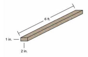
Each furring strip is 6 feet (1.8 m) in length, so if you are covering a small area of damage, one strip may suffice. If you are covering a large area, you may need to abut two or more strips until you have a long enough length of wood.
