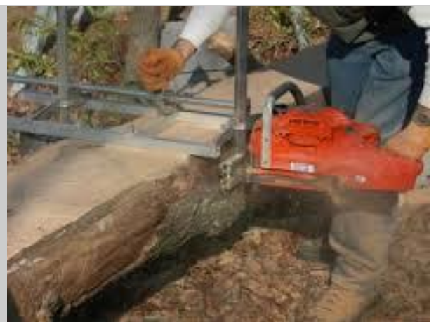
Frame for chainsaw yields higher quality lumber.
