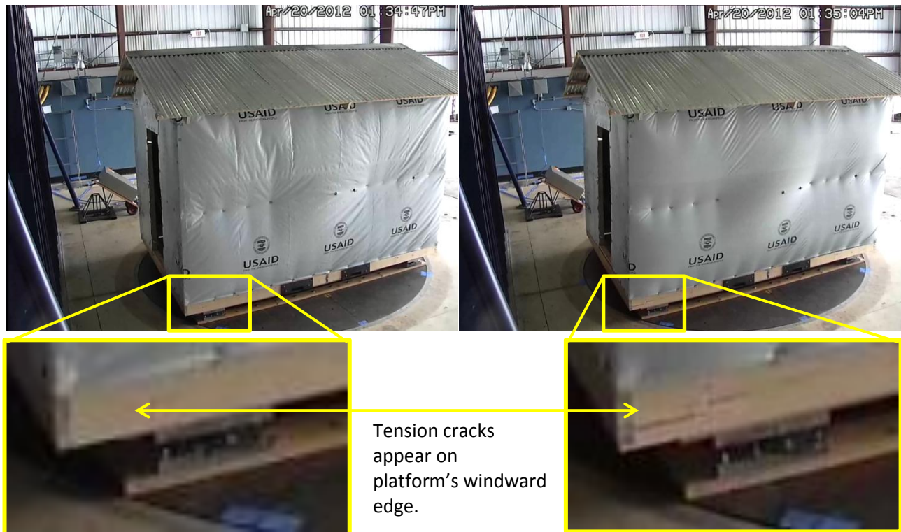
Figure 28 - Tension cracks on T-shelter base platform's windward edge
