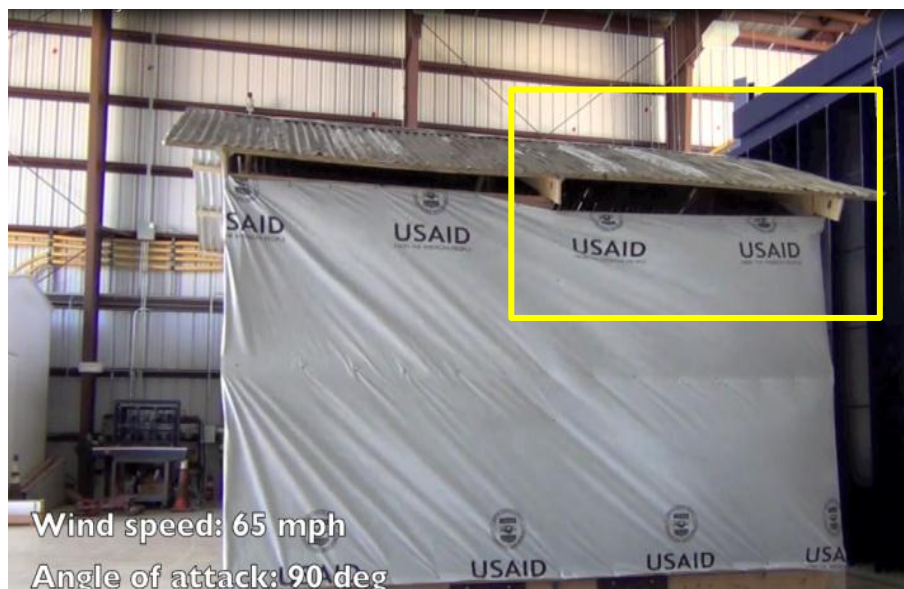
Figure 22 – T-Shelter 1 test at 65 mph and 0° and 90°; some of the wood boards part of the framing detached
