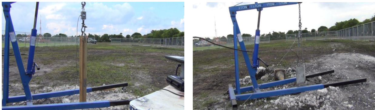
Figure 15 – Pull-out test of footings with hydraulic jack. Left: 4x4 embedded in concrete, right: precast concrete pier
