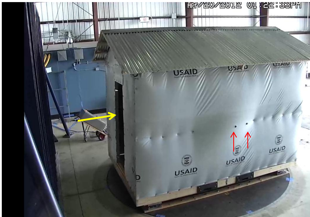
Figure 27 - T-Shelter 2 door failure at 85 mph and 90 degrees. Red arrows show OFDA plastic perforated by tin caps
